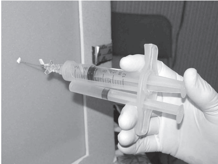
Figure 1. Method for measurement of physician control of needle and syringe: with the reciprocating syringe held with one hand, the foam target is shown just anteriorly. The rigid polystyrene marker is placed on the needle to a preset indelible mark on the needle shaft, and then the needle is advanced into the target tissue until the polystyrene marker is touching the surface of the target tissue. The physician operator then performs the syringe procedure. Loss of control in the forward direction (ie, unintended penetration) pushes the polystyrene marker posteriorly on the needle shaft past the indelible mark, permitting precise measurement of loss of control in the forward direction. Loss of control in the reverse direction (ie, unintended retraction) lifts the polystyrene marker off the surface of the target tissue, exposing a length of the needle shaft, permitting precise measurement of loss of control in the reverse direction (ie, retraction).
